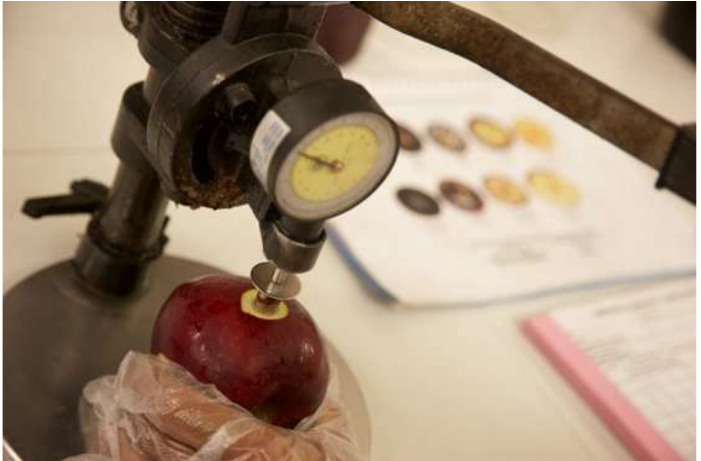
Figure 1: Skin Firmness Testing of Apples
